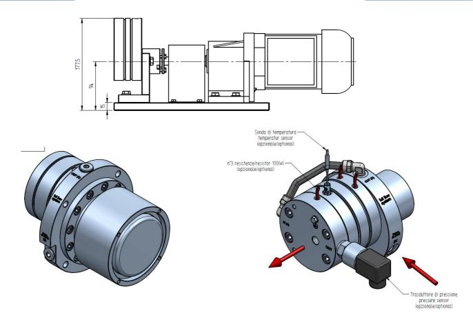
PLB pumps are designed with the basic pricriples of MVV but adding o-rings between the plates, to have the ability to handle viscosities under 100cP. It's fully made in Martensitic stainless steel with 54-56 HRC hardness.
